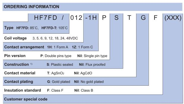
Notes: 1) Under the ambience with dangerous gas like H<sub>2</sub>S, SO<sub>2</sub> or NO<sub>2</sub>, plastic sealed type is recommended; Please test the relay in real applications. If the ambience allows, flux proofed type is preferentially recommended.
